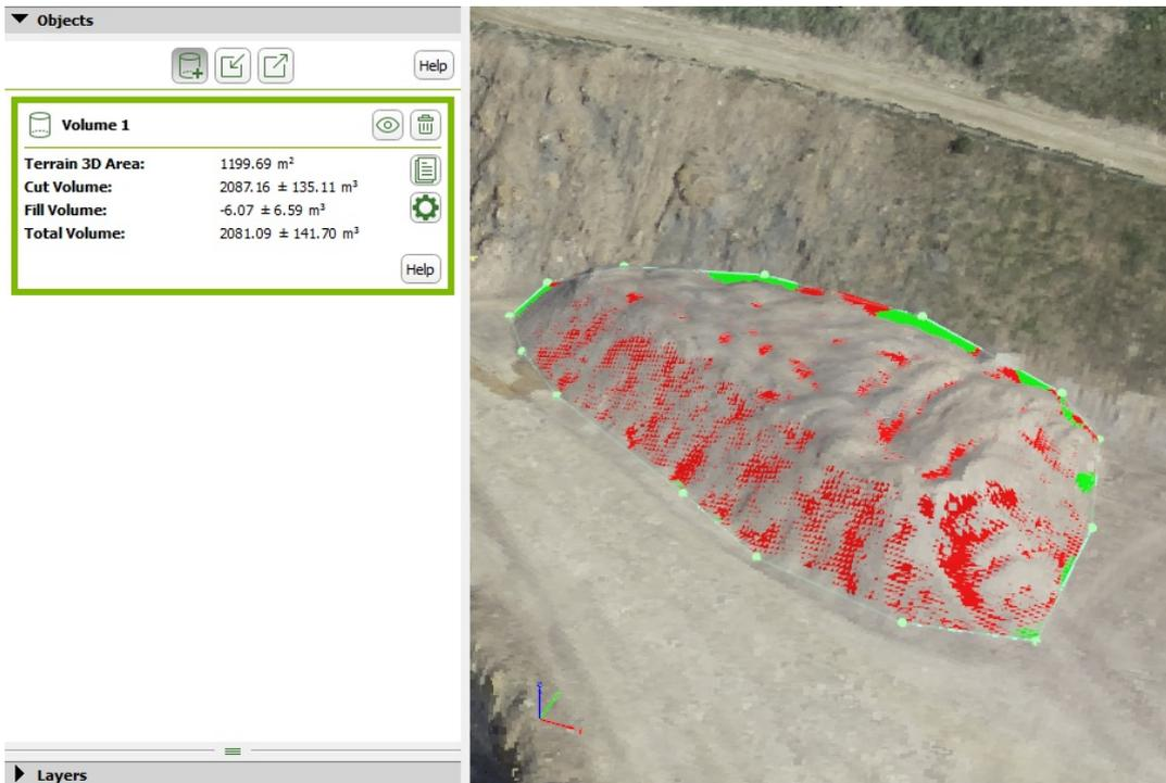
The screenshot shows a software interface with a sidebar on the left and a 3D terrain view on the right. The sidebar, titled "Objects", contains a table of volume data for "Volume 1". The table lists the following values:
