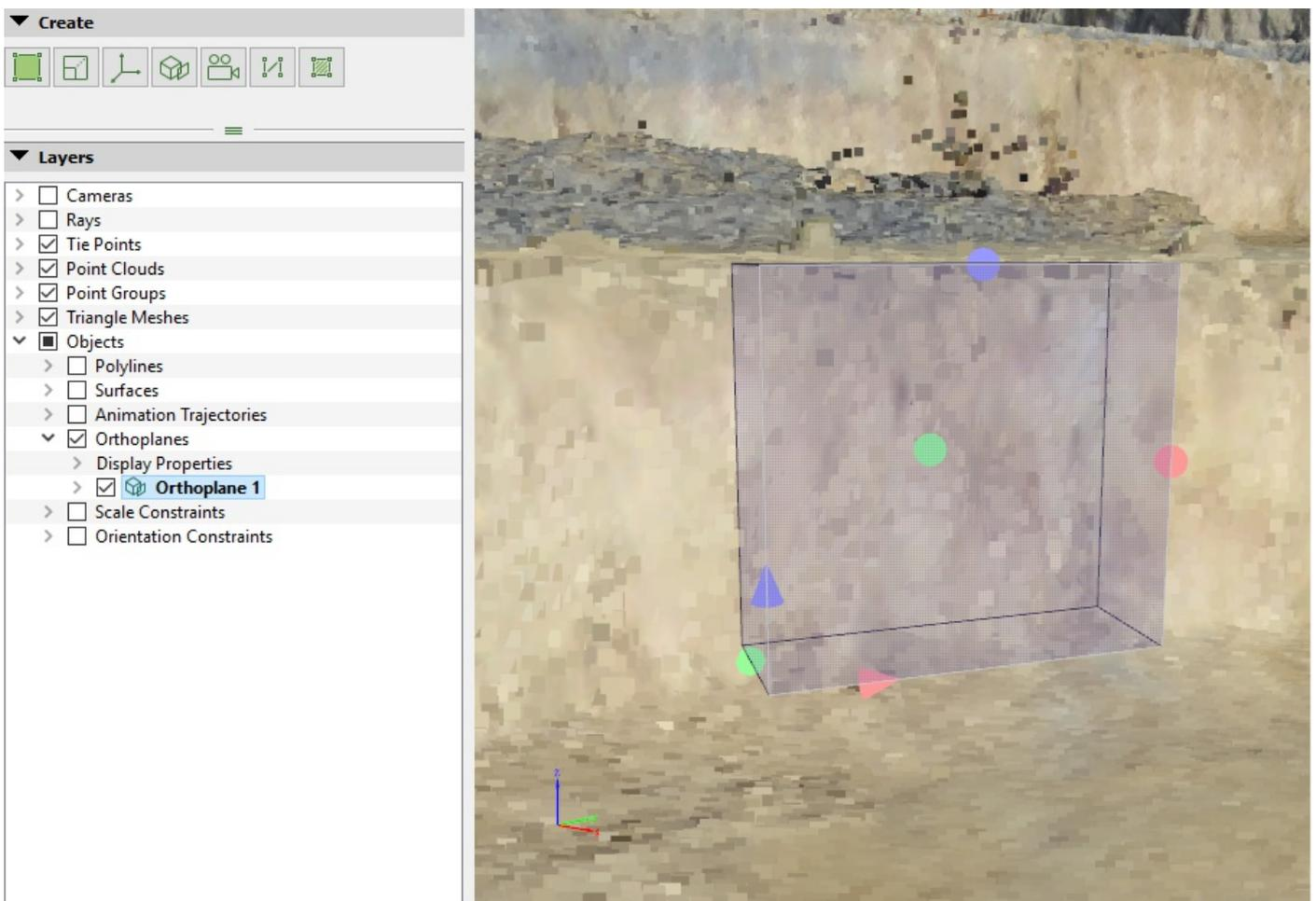
Contains the list of orthoplanes added to the project. An *Orthoplane* is a tool to create one or several orthophotos of arbitrary areas of the model without having any impact / modifications in the model.
