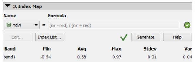
The screenshot shows the '3. Index Map' window. The 'Name' dropdown is set to 'ndvi' and the 'Formula' field contains '(nir - red) / (nir + red)'. A green checkmark icon is visible next to the formula. Below the formula field are buttons for 'Edit...', 'Index List...', 'Generate', and 'Help'. A green checkmark icon is also visible above the 'Generate' button. At the bottom, there is a table with columns: Band, Min, Avg, Max, Stdev, and Var. The table content is as follows:
