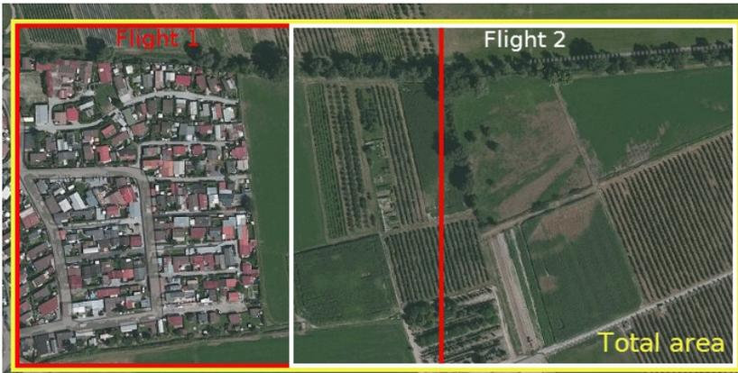
Figure 6. Recommended image acquisition plan for 2 flights.
